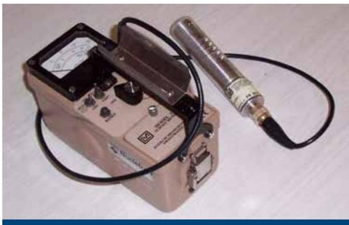
Portable radiation detection instrument
