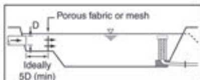
Figure 5(b) – Typical layout of inlet chamber with opposing inlet pipe (Type C basin)
