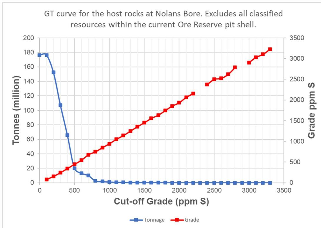
Figure 2—1 Grade tonnage curve for sulfur
