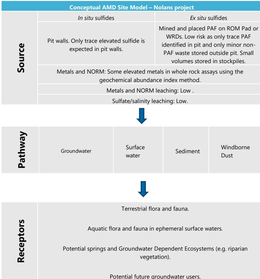
Figure 3—2 Nolans Bore AMD and NORM Conceptual Site Model
