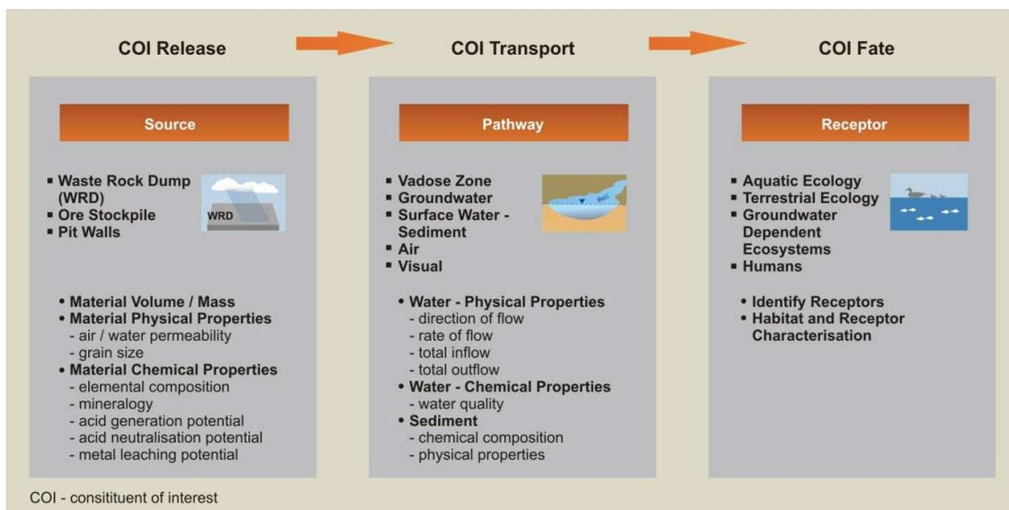
Figure 3—1 The AMD Source→Pathway→Receptor Model (INAP, 2011)
