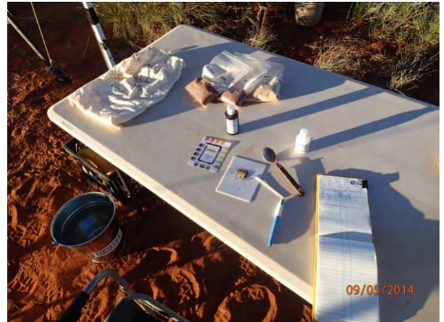
Soil samples were taken during drilling all the NE Southern Basins Bore for field pH testing and depot salinity testing. A set of soil samples were collected in chip trays and plastic sample bags for the soil sample library.
