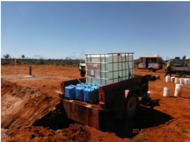
Flushing out plastic water sample drums
