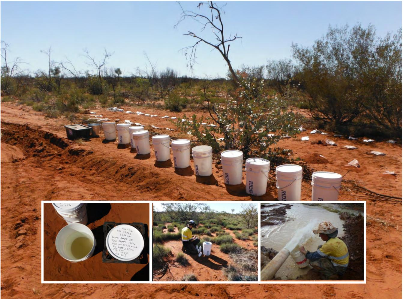
A large number of drilling water samples collected at the end of the bluey line were field tested to provide an indication of the water quality changes with depth drilled.
