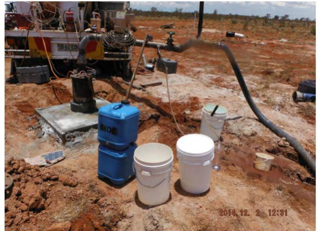
Isotope water samples taken in 20 L blue drums at end of constant rate test
