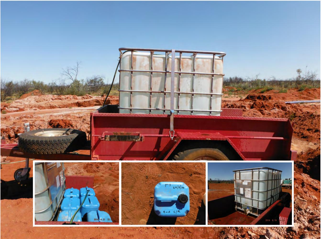
Bulk water sample (1000 litres) taken from RC # 22 (PB1) for ore metallurgical testing, pod flushed using pumped groundwater. Twenty litre plastic drums being flushed for isotope water sample testing.
