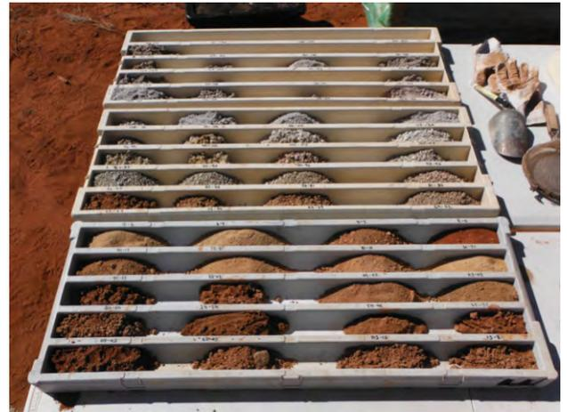
Grab strata samples were taken during drilling all the NE Southern Basins Bores at 3 m intervals. Representative sets of strata samples were placed chip trays and plastic sample bags for the *Arafura* strata sample library.
