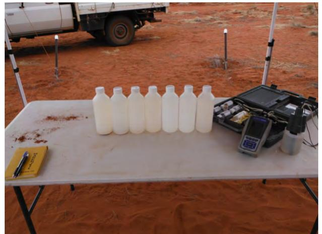
20 L bucket water samples were taken every rod (6m) following intersection of aquifers. EC, pH, T & OH were measured in the field and from these analyses buckets were selected for standard chemical and trace metal laboratory analyses after the sediment had settled. The samples were then placed in ice and remained in refrigeration until analysed in the Darwin NTEL Laboratory.
