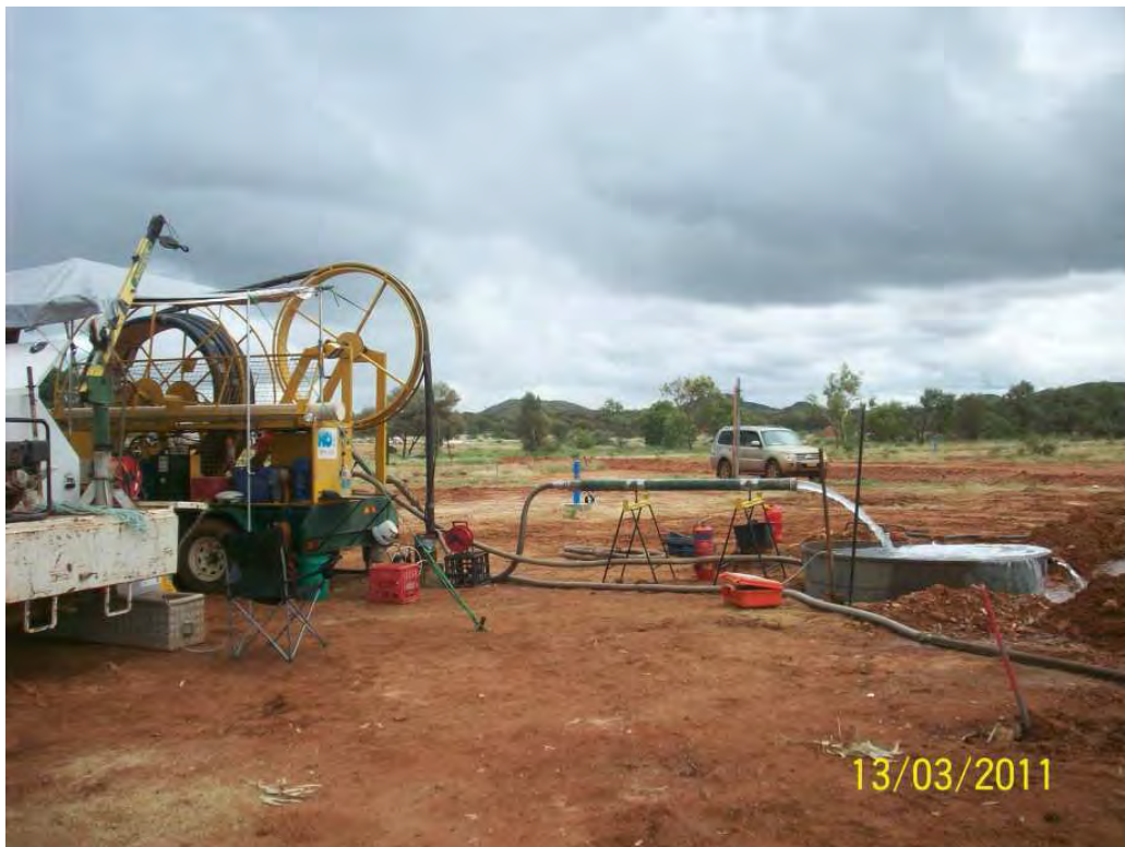
Photograph 4: pumping test setup
