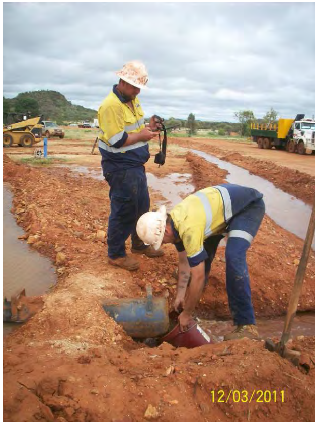
Photograph 3: Measuring yield using 20L bucket and stopwatch
