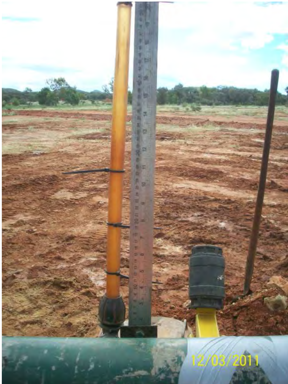
Photograph 5: circular orifice weir piezometer tube and scale
