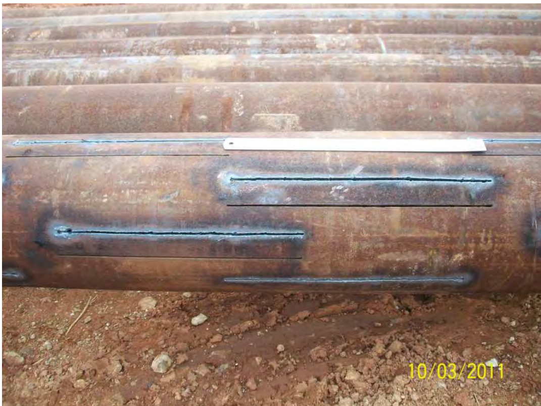
Photograph 2: Mild steel slotted casing with additional oxy-cut slots for increased open-area
