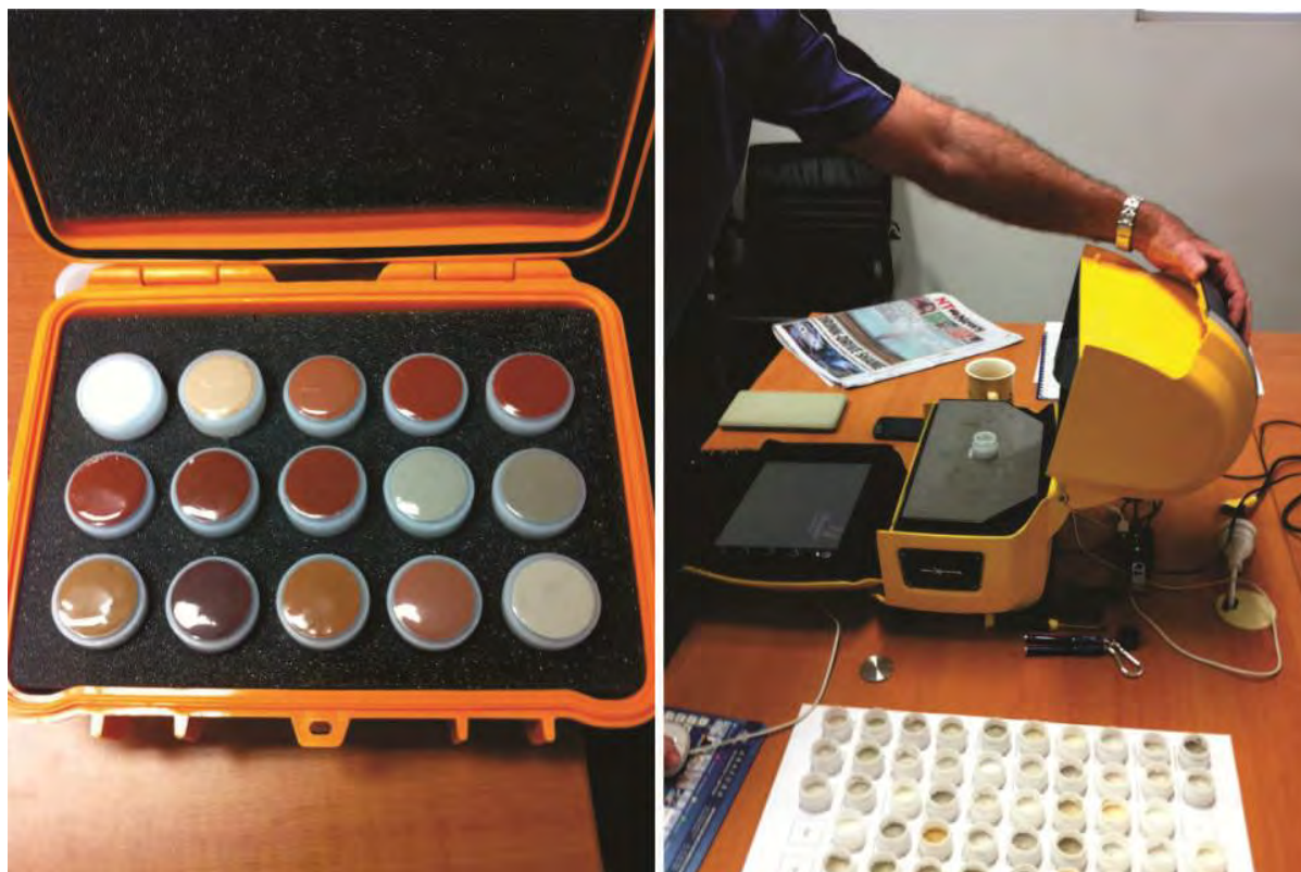
Figure 1 Left: The certified standards starting with A in the top left and finishing with O in the bottom right of the box. Right: The Olympus X-5000 Series Mobile XRF unit with a batch of pulps pressed into the sample cups on the numbered sheet. Also notice the stainless steel calibration disc to the right of the pXRF
