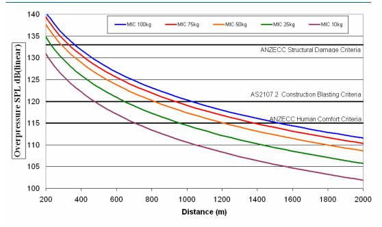
Figure 14-1 Airblast overpressure predictions for different charge masses and distances
