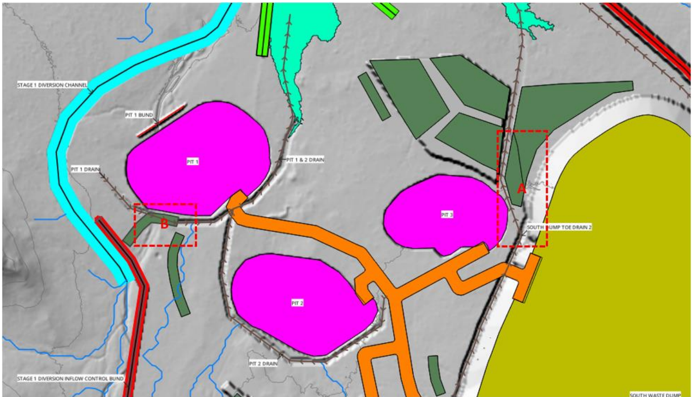
Inset 8: Clashes between the hydraulic model and the 50% level of design: Pit area of the Stage 1 mine layout.
