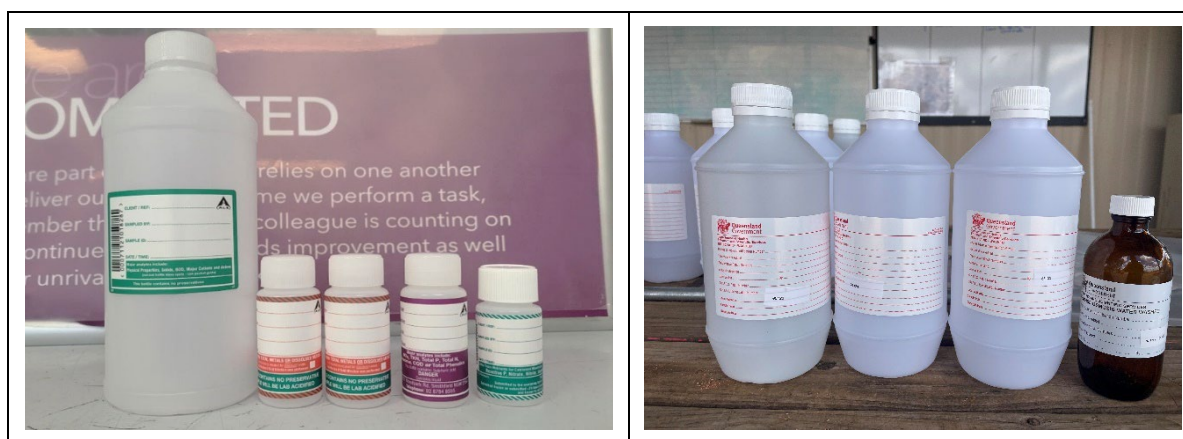
Figure 2—1 Example of bottle set prepared for: general parameters (left); and radionuclides analysis (right).
